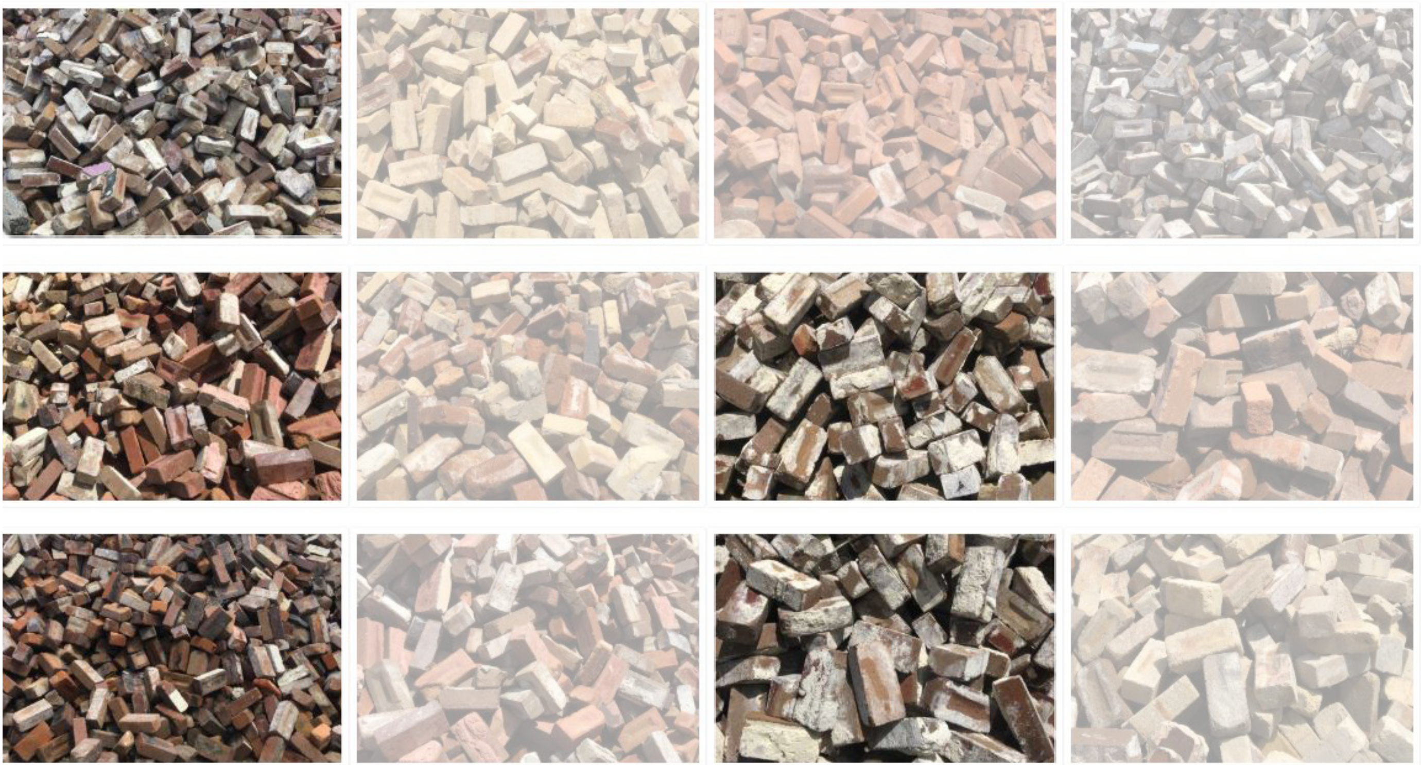
Sydney brickwork has a series of tonal variations depending on the location of the quarry. Brickwork within the Ashbury conservation area is typically sourced from Wianamatta shale. The proposed brickwork will be consistent with this existing stock.
